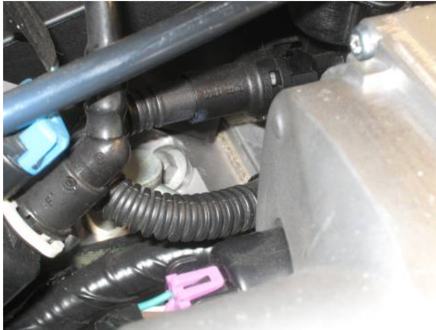
Figure 4: PCV Line Intake Plenum Connection
