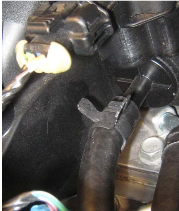
Figure 6: Rubber Hose Installed on PCV Inlet (To Side of Catch Can)
