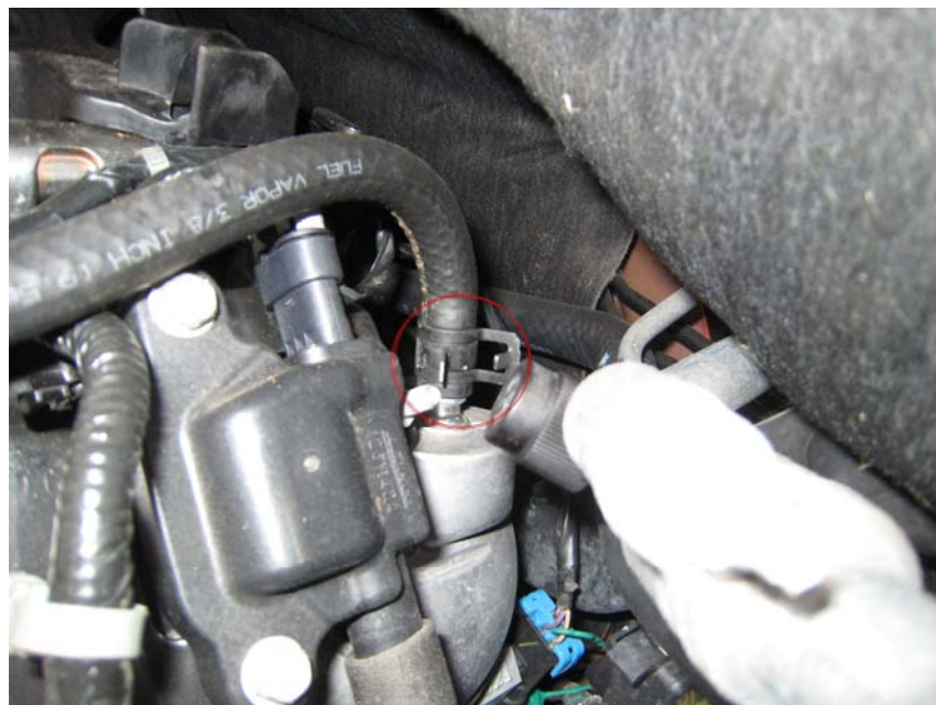
Figure 5: PCV Line Engine Outlet Connection (Circle for Clarity)
