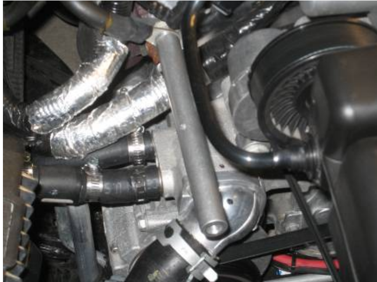
Figure 2: Aluminum Rod Secured to Engine Block
