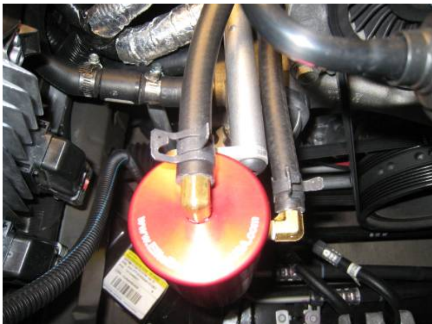
Figure 9: Hoses Installed on Catch Can
