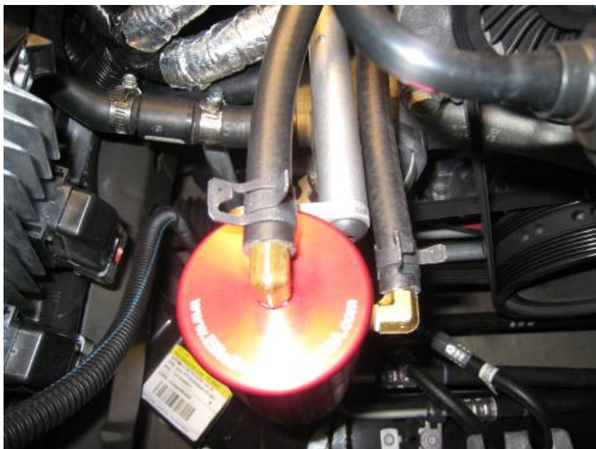
Figure 9: Hoses Installed on Catch Can
