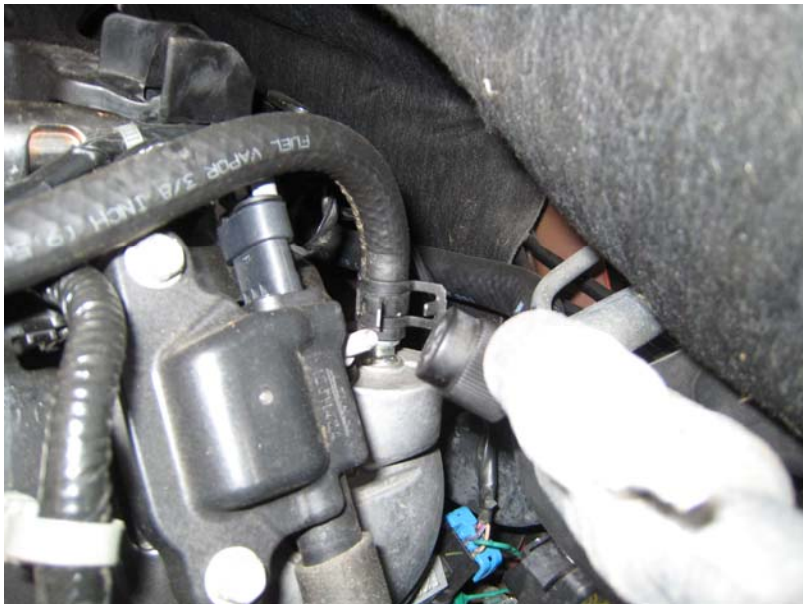
Figure 7: Rubber Hose Installed on PCV Outlet (To Top of Catch Can)
