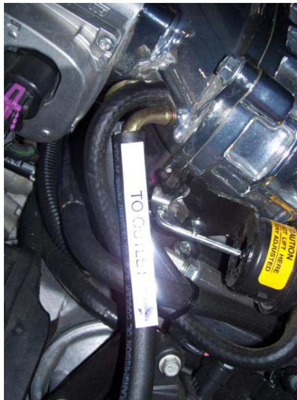
Figure 10: Supercharger Inlet Connection (Routes to Outlet on Catch Can)
