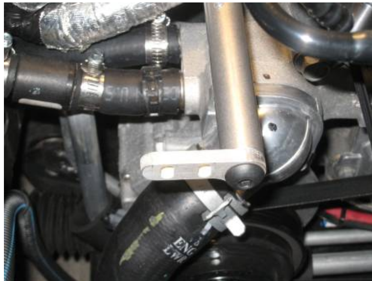
Figure 3: Bracket Installed on End of Rod
