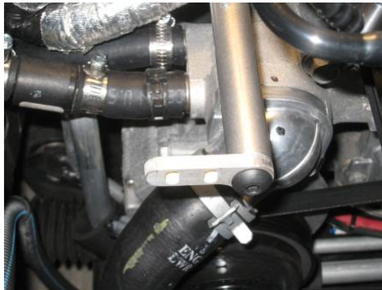
Figure 3: Bracket Installed on End of Rod
