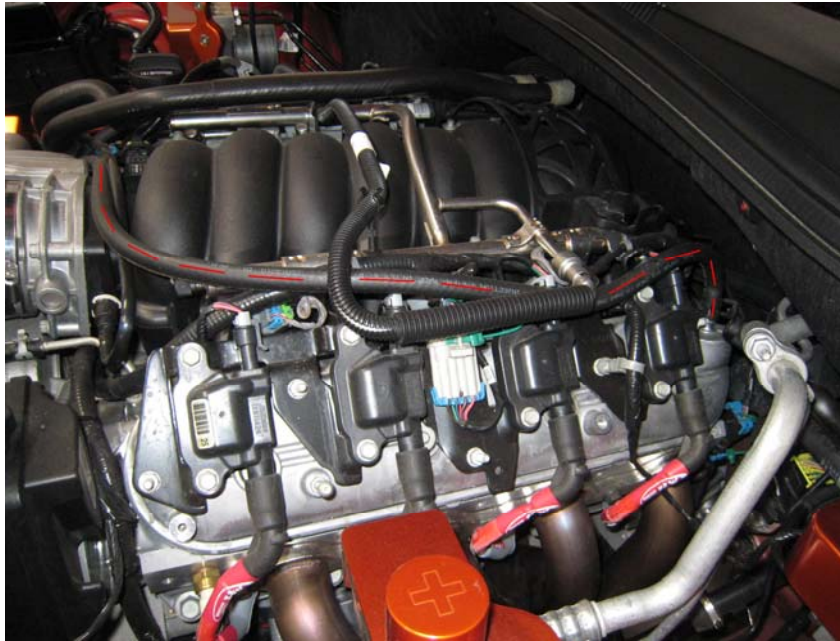
Figure 8: Hose Routing from PCV Outlet (Line Highlighted in Red for Clarity)
