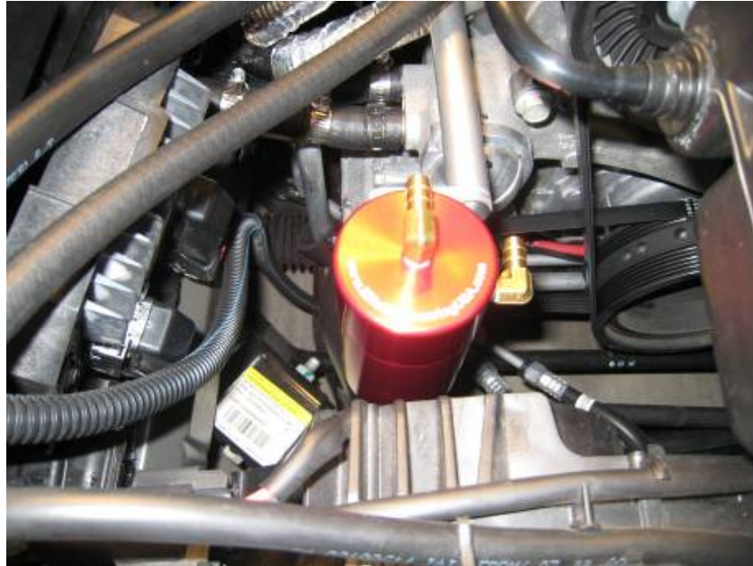
Figure 7: Catch Can Installed on Bracket
